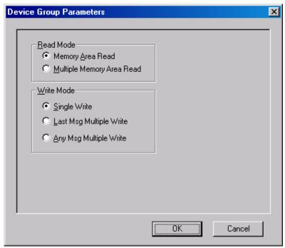
The Device Group parameters dialog can be used to configure preferred Read mode and Write optimization mode.
